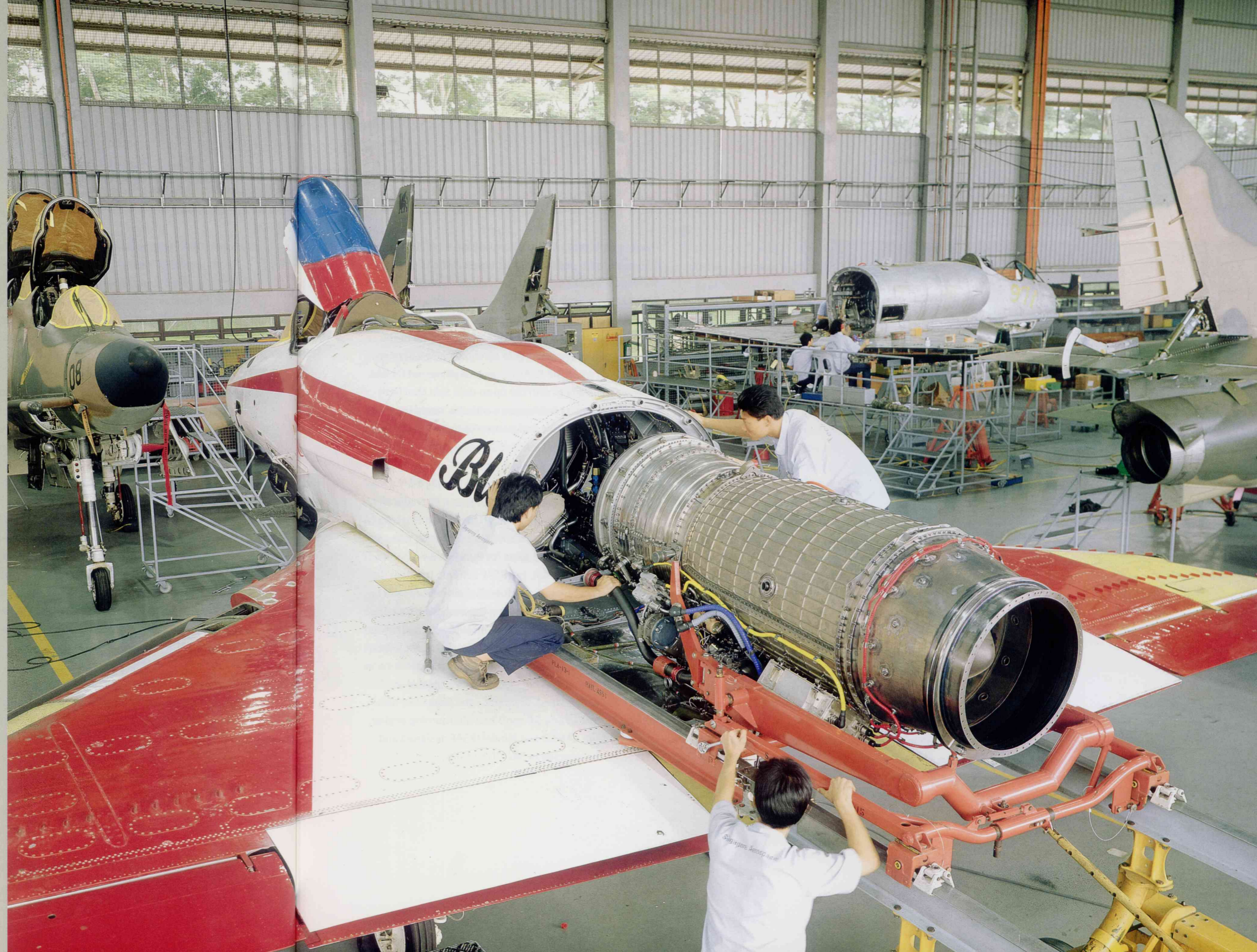
Installing the F404 engine into a Super Skyhawk.
