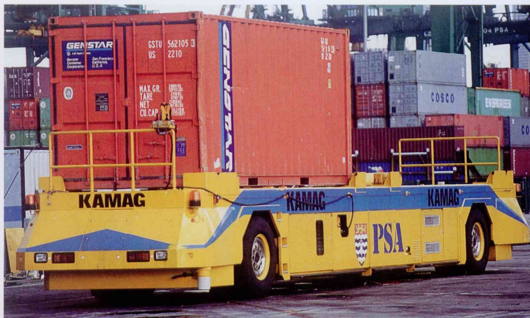
An Automated Guided Vehicle (AGV) at work in Singapore's busy harbour. The AGV is a project of CEI Technologies, an ST subsidiary.
