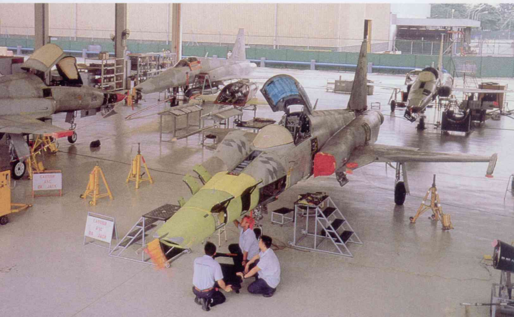
A typical day at the ST Aero hangar: fixing up the F-5E IIs.
