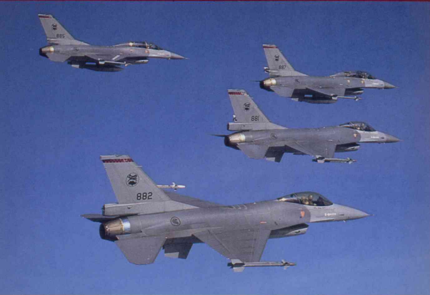
The RSAF's premier fighter-interceptor, the F-16. Instead of a conventional array of instruments and controls, the F-16 has a sophisticated head-up display (HUD) and a fly-by-wire control system. This allows the pilot to fly with a minimum of physical movement and a maximum of attention to combat, since he no longer has to look down to check his control panels. Such state-of-the-art interfaces between man and machine have become essential to modern weapons systems.
