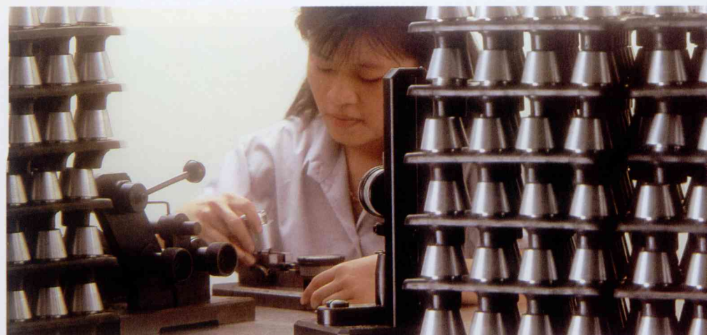
Worker at CIS assembling fuses.
