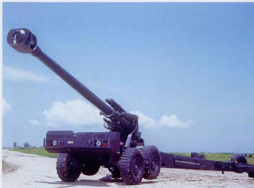
The FH 2000, a 52 calibre 155mm field howitzer, boasts state-of-the-art capabilities and performance, and can fire all NATO-type ammunition. Developed by ODE, the FH 2000 is the company's third generation field howitzer, based on the earlier FH 88.
