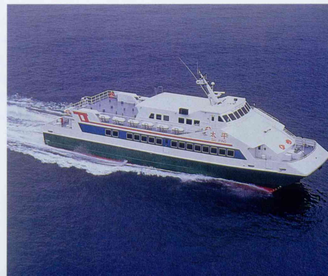
The “Tai Ping”, a 282-passenger high speed catamaran ferry built by ST Shipbuilding. The vessel is owned by Dong Guan City Humen Hong Kong/Macau Passenger Ferry Co.
