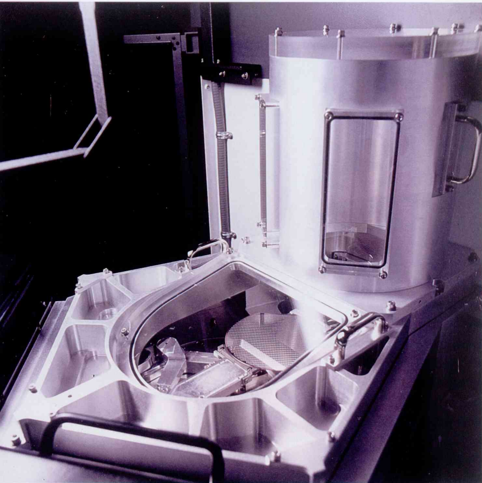
A cluster tool used for oxide or metal deposition in the thin film section of the fabrication process.
