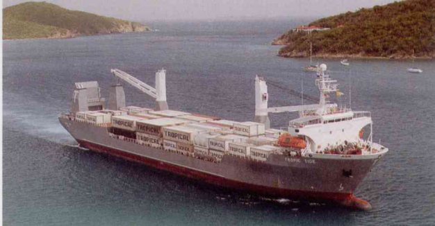
The "Tropic Tide", a 400 TEU RoRo/LoLo type Container Vessel built by ST Shipbuilding. The ship, built in 1993, has received strong praise from its owner, the US-based Tropical Shipping & Construction Company.
